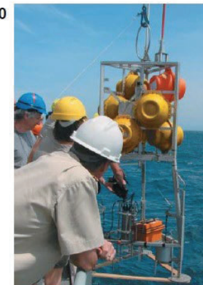
Figure 22.21 Deployment of deep-sea lander. The lander is equipped with a bank of microelectrodes to measure distribution of chemicals in marine sediments.
